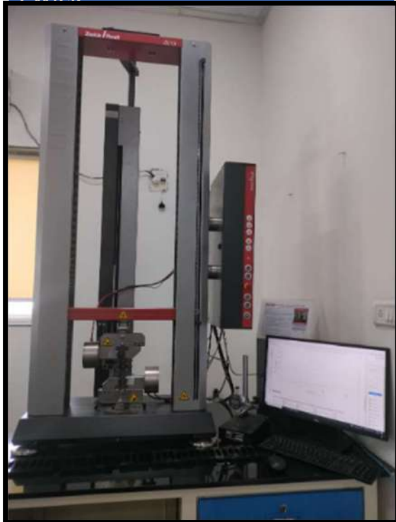
Universal Testing Machine Zwick
