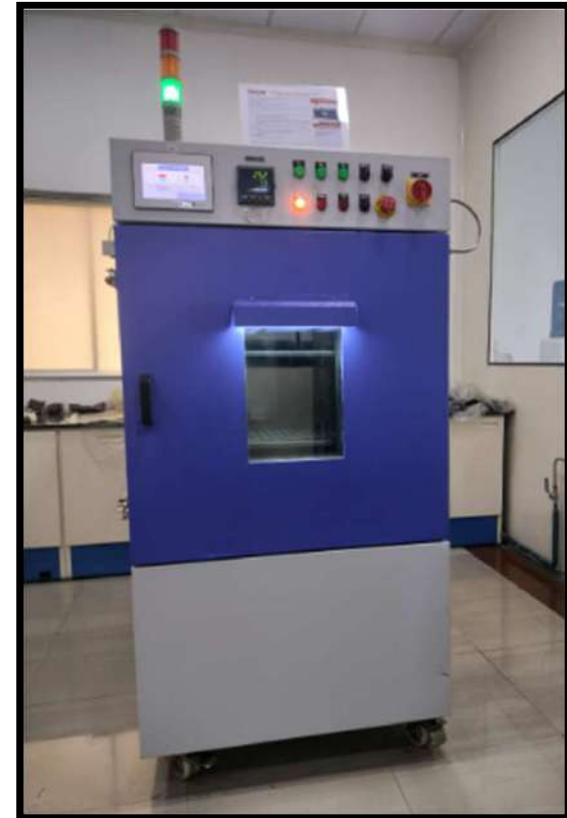
Temperature & Humidity Chamber
