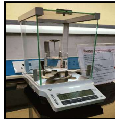
Specific Gravity Balance
