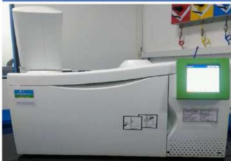
Gas Chromatography (Clarus-590) Perkin Elmer
