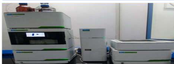
High performance liquid chromatography (LC-300) Perkin
