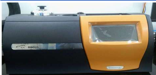
Differential scanning calorimetry (DSC) TA MAKE - DSC-25
