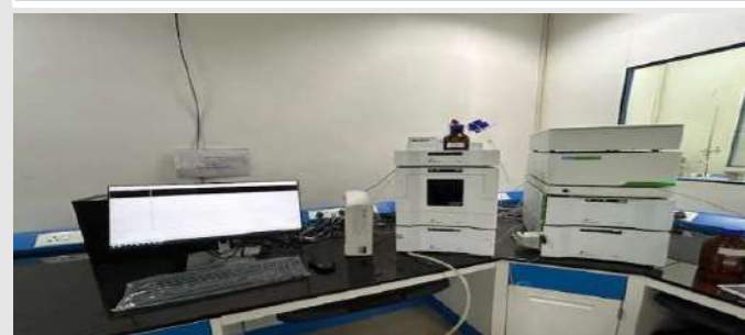
Size Exclusion Chromatography (SEC) GPC For Molecular weight Determination of Resin
